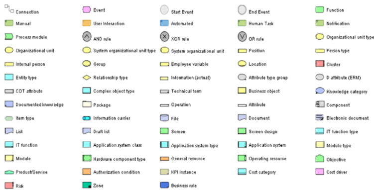
FIGURE 24: ELEMENTS OF EVENT-PROCESS-CHAINS (EPC) AND PROCESS-CHAIN-DIAGRAMS (PCD)
